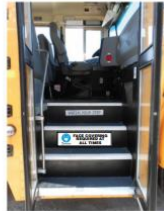
Measurement for School Bus step riser is 6.5" tall by 24" wide.
